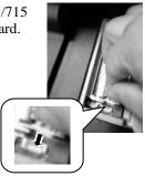
5. Determine that the USB I/O cable is securely connected to the cable connector of the main board.
