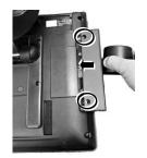
9. Fix the SA-705/715 onto the terminal with the two fixing screws.
